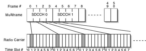
Fig. 5. Timeslot 1 from each frame in a multiframe creates the logical SDCCH channel. In a single multiframe, up to eight users can receive SDCCH access.
