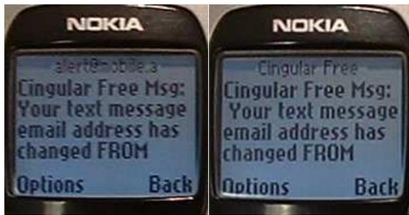
Fig. 6. Spoofing a service provider notification is trivial due to interface and message length constraints; the left image is a forgery of a legitimate service notification (right) provided by Cingular (Note the top line).
